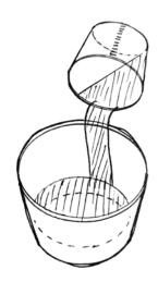
Step 1: Mix and pour white resin into mould. Repeat with blue resin
